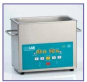
Keypad with digital LED panel for simultaneous display for set & actual temp. and set & actual time.
