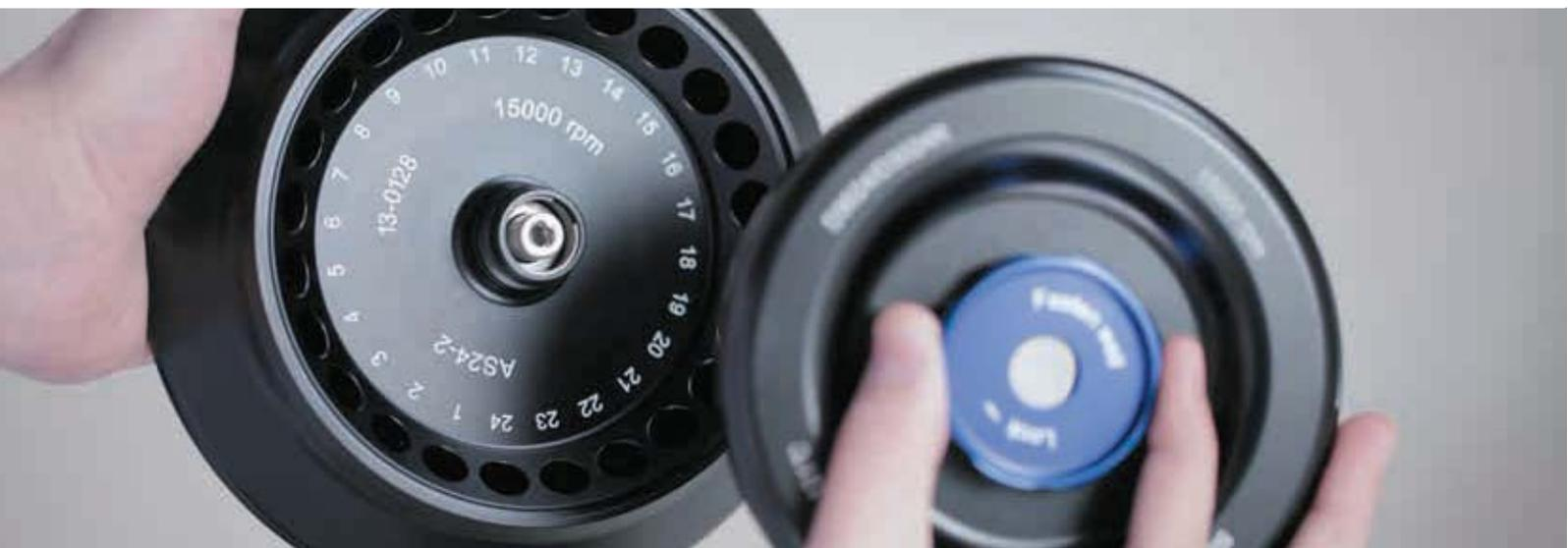
D/LAB hematocrit centrifuge with AC24P hematocrit rotor is used for determination of volume fractions of erythrocytes in blood for diagnostic purposes and doping tests. Also it is used for the photometric determination of bilirubin content in neonate blood samples. Hematocrit centrifuge with A24-2P tube rotor, can be used for extraction of DNA and RNA.
